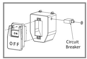
**Figure 6.** Location of switch circuit breaker.
